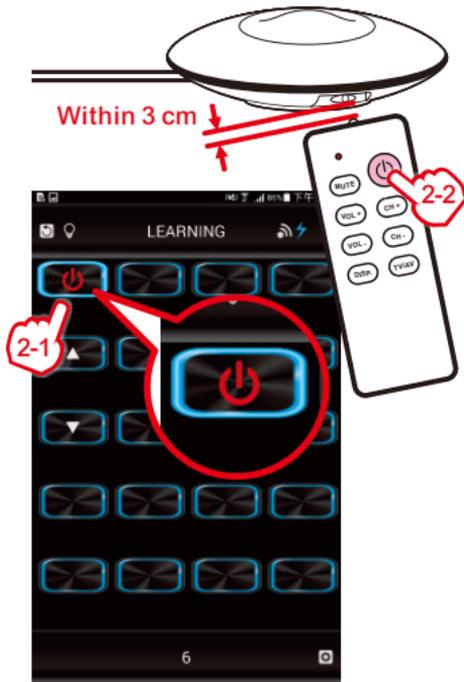
2. Move your remote control close to the indicator of control box and press "POWER" button on the remote control. If it learns successfully, the "POWER" button in the app will be framed in BLUE.
