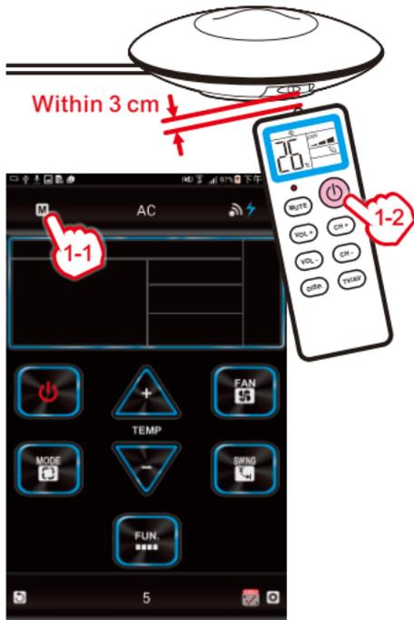
1. Turn off the air-conditioner Select "AIR-CONDITIONER MODE" Press "M" to starting match Connect the infrared receiver between air-conditional remote controller and control box within 3 cm Press "Power". i-Ctrl will start to match the suitable code for the air-conditioner around few minutes.
