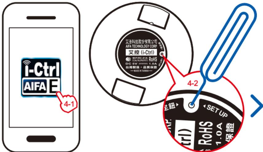
4. Please star "AIFA i-Ctrl" app from smart phone or tablet; Use the paperclip to press the "SET UP" button.
